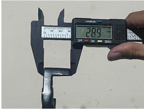
Gambar 4-39 Pengukuran Panjang *Trigger Switch* Rem Asli
