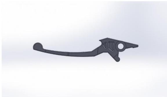
Gambar 4-12 Desain *Lever Brake* Yamaha Nmax
