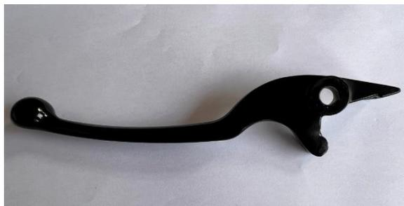
Gambar 4-9 Lever Brake Original Yamaha Nmax
