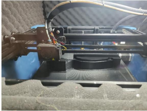
Gambar 4-21 Proses *3D Print Molding*
