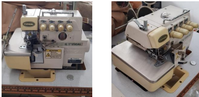
Gambar 3.5 Mesin Jahit Obras 4 Benang Typical Progressive
