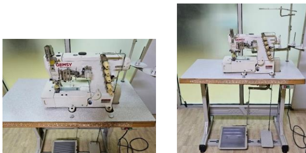
Gambar 3.6 Mesin Jahir Overdeck
