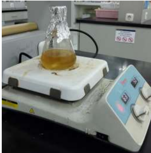
Gambar 3. 5 Proses Wet Peroxide Oxidation Sampel (WPO)
