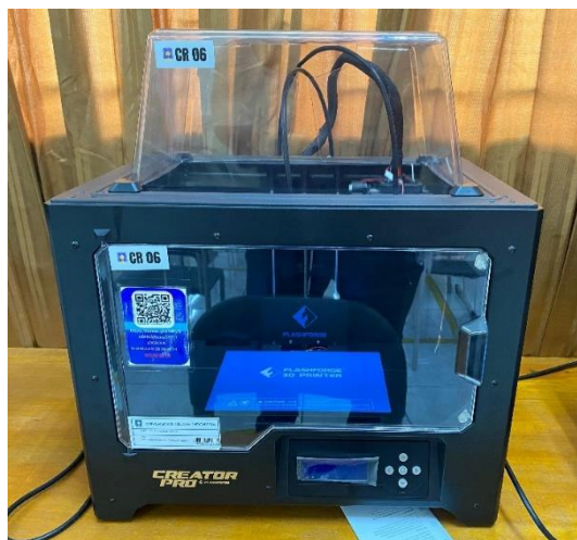
Gambar 2- 2 Mesin 3D Print FDM ( Fused Deposition Modelling )
