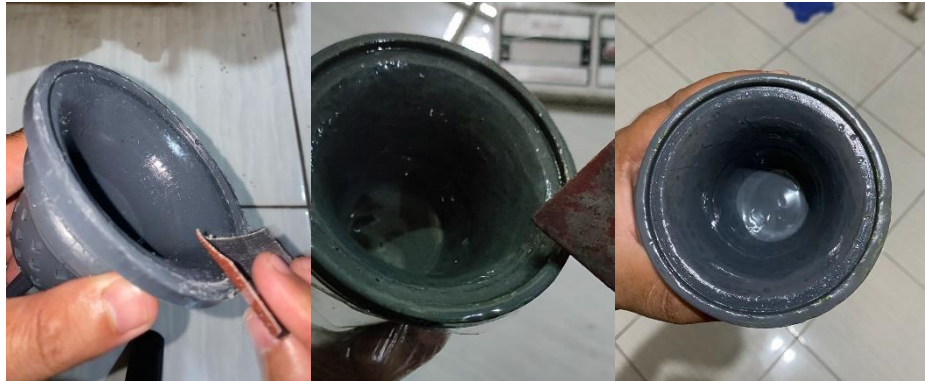
Gambar 4- 29 Proses finishing komponen Stupa Candi Borobudur
