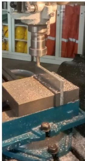
Gambar 4. 29 *Facing* Bagian Samping Aluminium
