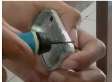
Gambar 4. 60 Proses *Deburring*
