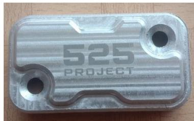
Gambar 4. 62 Hasil Laser *Marking*
