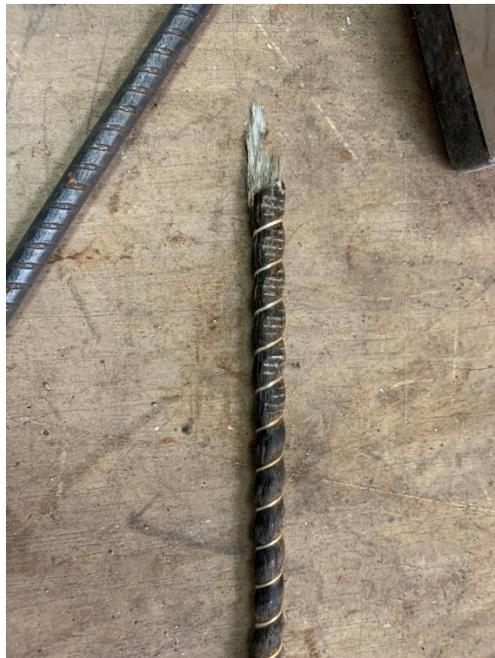
**Gambar L-6.2 Tulangan Basalt Yang Patah**
