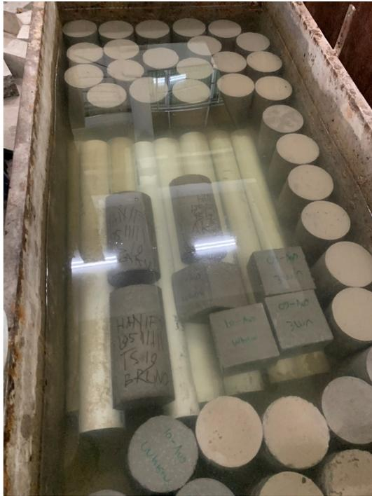
**Gambar L-9 Perendaman Silinder Beton *Trial***
