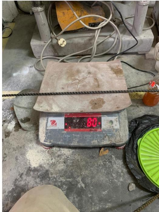
**Gambar L-5.1 Pengukuran Berat Tulangan Basalt Tidak Korosi**
