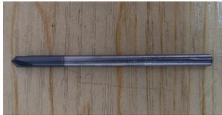
Gambar 3.9 Mata pahat *Chamfer* 3 mm
