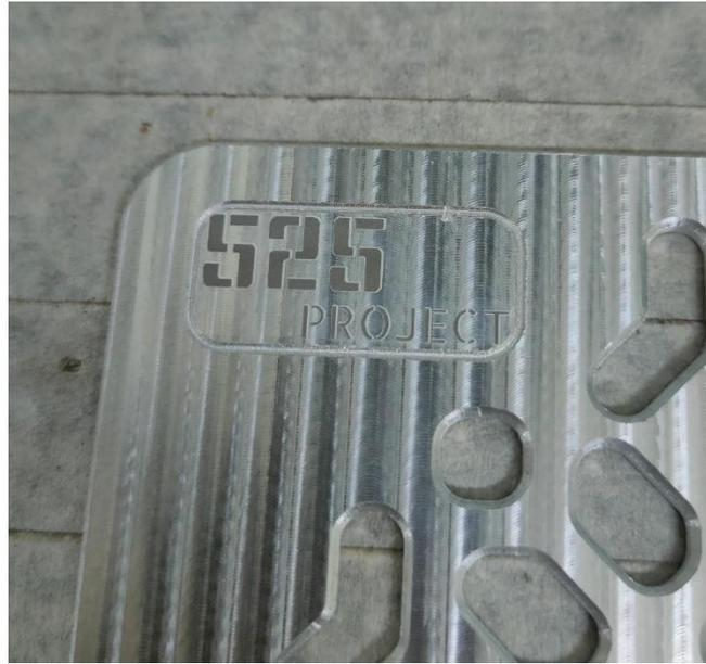
Gambar 4- 50 Hasil laser *marking*
