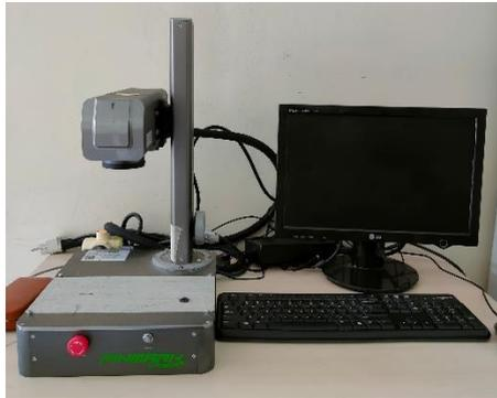
Gambar 3- 5 Mesin laser *marking*
