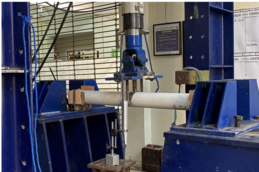
Gambar 4.16 Setting Pengujian Lentur
