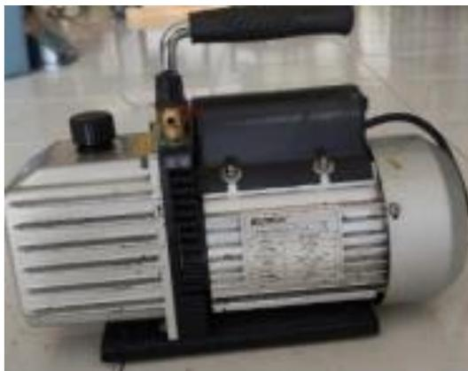
Gambar 3-13 Pompa Vakum
