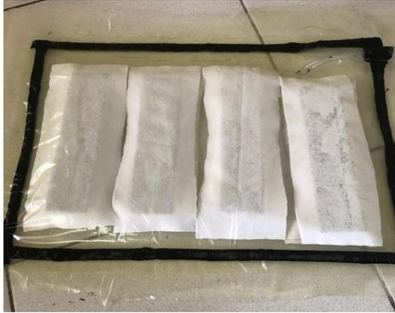
Gambar 3-32 Rangkaian *Vacuum Bagging*
