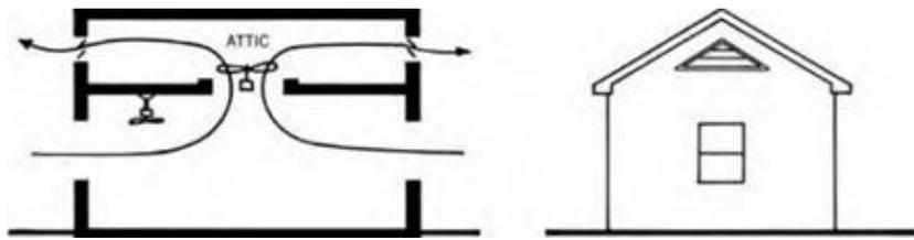
Gambar 2.42 Sistem cross ventilation
