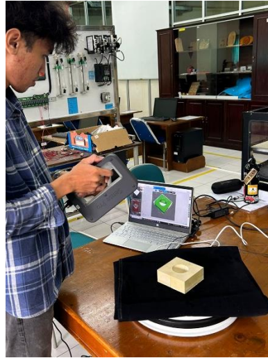
Gambar 3-28 Proses 3D Scanning
