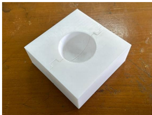
Gambar 4-3 Hasil Proses 3D Printing Puzzle Mold
