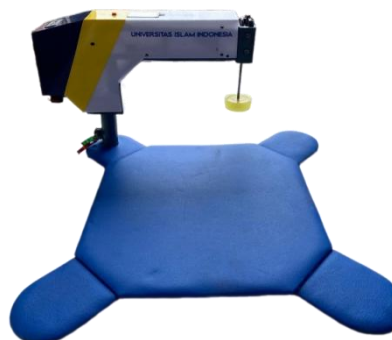
Gambar 4 - 16 Alat RJP otomatis final .
