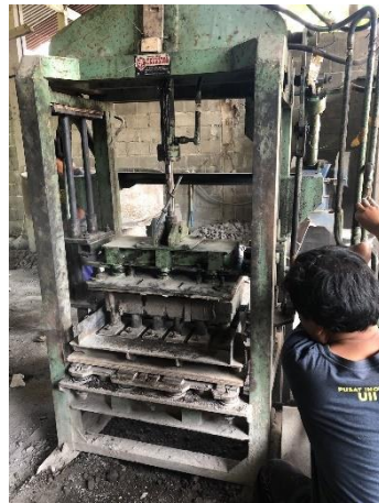
Gambar L-3.2 Proses Press Paving Block
