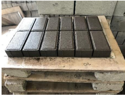
Gambar L-3.3 Hasil Proses Press Paving Block
