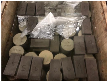
Gambar L-4.4 Proses Perendaman Pengujian Daya Serap Air Paving Block
