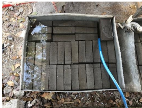
Gambar L-3.4 Proses Perendaman Paving Block
