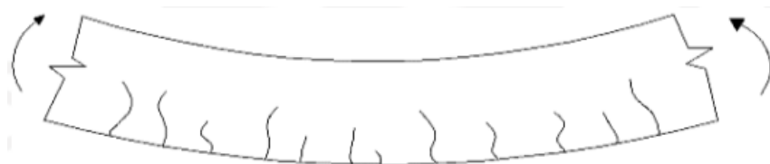
Gambar 3. 11 Retak Lentur Murni (Sumber: Kholilul dkk, 2009)
