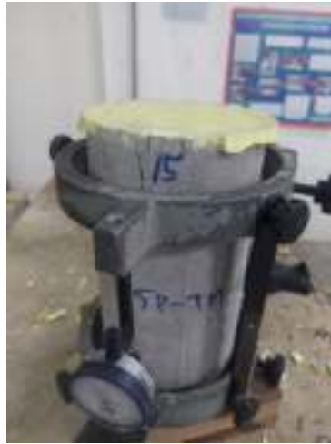
Gambar 5.15 Benda Uji Dipasang Dial Gauge
