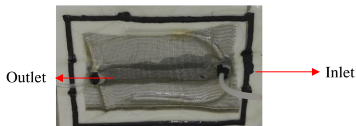
Gambar 3-44 Uji Coba Vaccum Infusion
