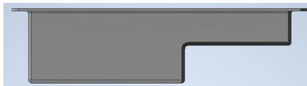
Gambar 4.2 Tampak Depan Desain Kitchen Sink
