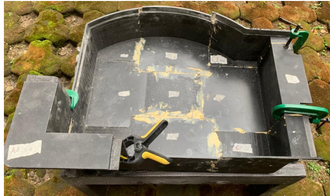
Gambar 4.10 Proses Puzzling Bagian A, B, C 1-3 bottom
