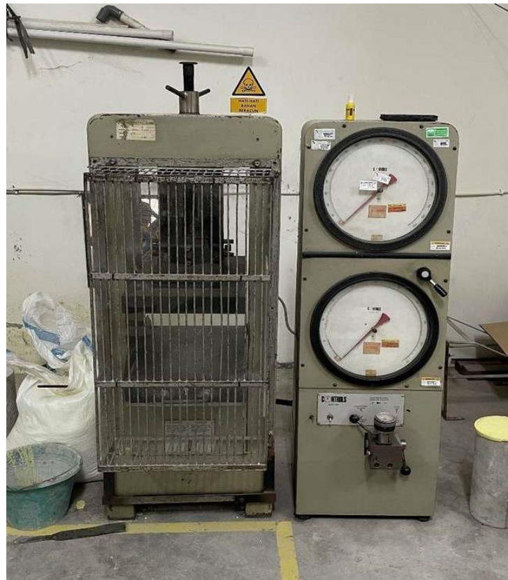
Gambar 4.1 Compressing Test Machine
