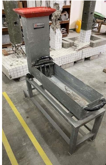
Gambar 4.6 Alat L-Shapped Box
