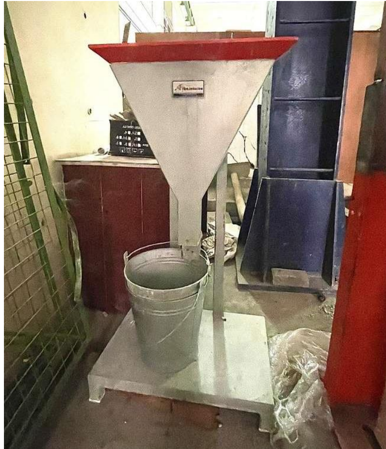
Gambar 4.5 Alat V-Funnel Test
