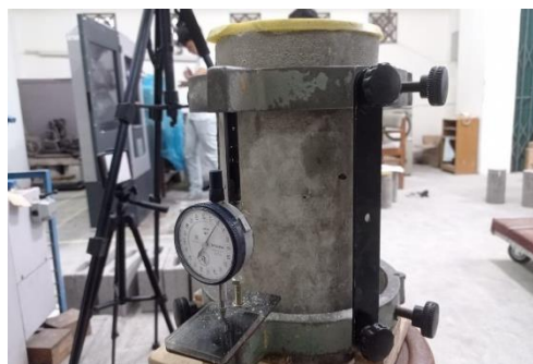
Gambar 5.19 Benda Uji Dipasang Dial Gauge
