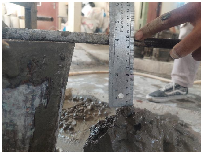
Lampiran 6.6 Pengujian Slump
