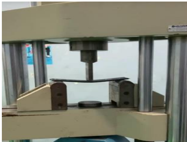
Gambar 3. 14 Proses Pengujian Bending
