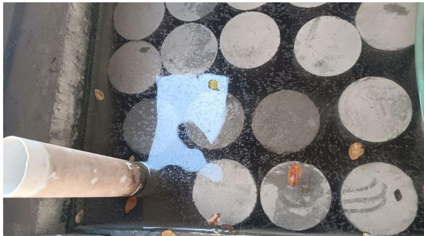
**Gambar L-10.4 Perendaman Beton Silinder**
