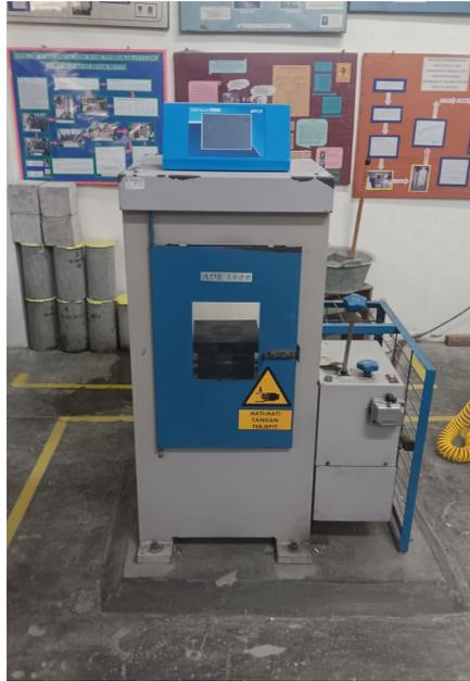
**Gambar L-9.12 *Compressive Test Machine***
