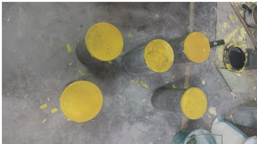
**Gambar L-10.5 Proses *Capping* Beton Silinder**
