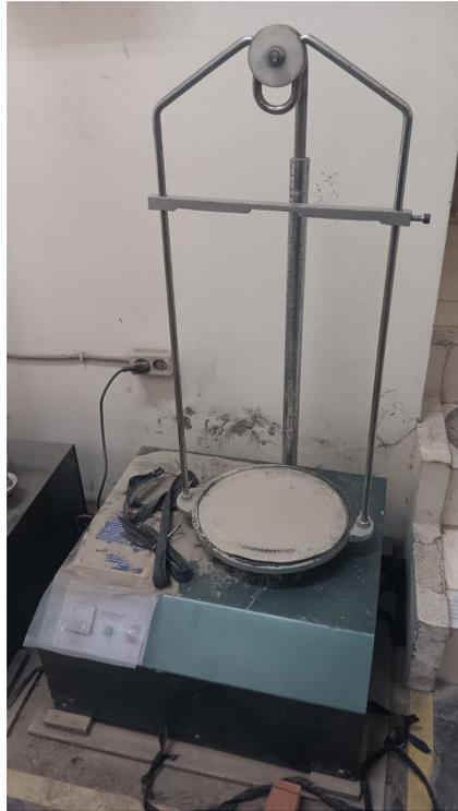
**Gambar L-9.10 Sieve Shaker Agregat Kasar**
