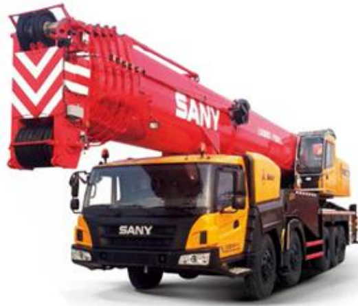
Gambar 3.6 Wheel Crane (SANY SCC1000E 100 ton Crawler Crane, 2017)
