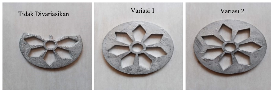
Gambar 4. 21 Hasil Spin Casting 700 RPM Percobaan 3
