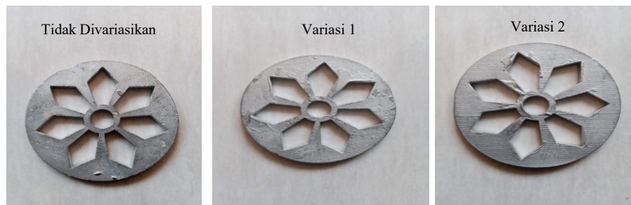
Gambar 4. 18 Hasil Spin Casting 600 RPM Percobaan 4
