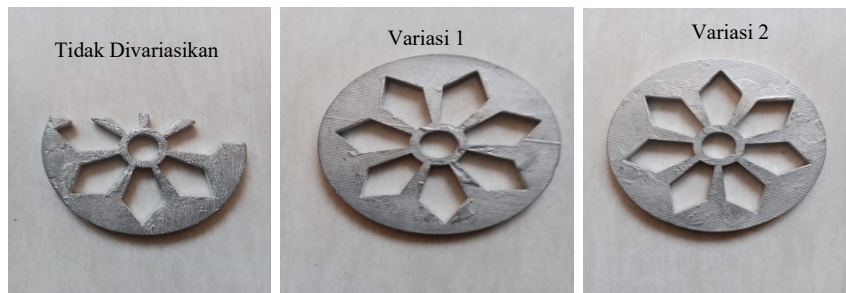
Gambar 4. 20 Hasil Spin Casting 700 RPM Percobaan 2
