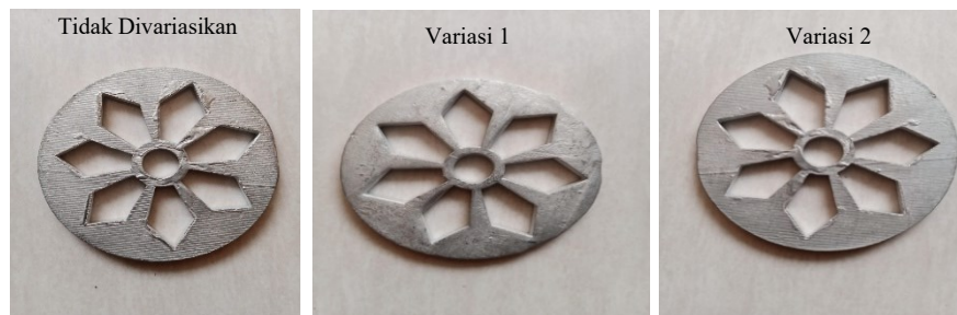
Gambar 4. 24 Hasil Spin Casting 800 RPM Percobaan 2
