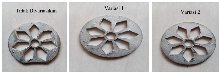
Gambar 4. 22 Hasil Spin Casting 700 RPM Percobaan 4
