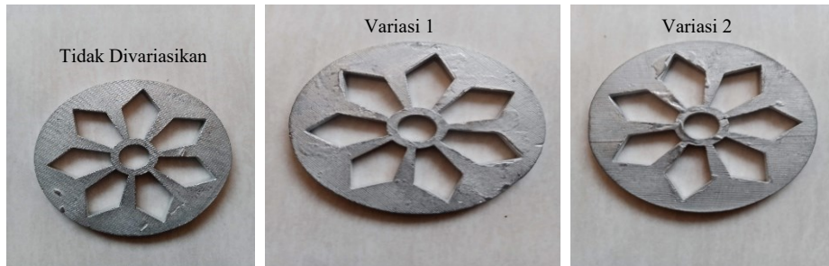
Gambar 4. 16 Hasil Spin Casting 600 RPM Percobaan 2
