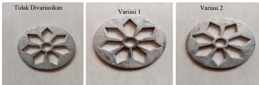
Gambar 4. 23 Hasil Spin Casting 800 RPM Percobaan 1
