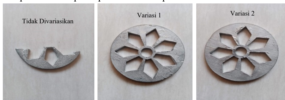
Gambar 4. 14 Hasil Spin Casting 500 RPM Percobaan 4
