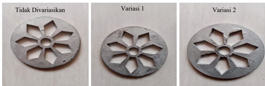
Gambar 4. 25 Hasil Spin Casting 800 RPM Percobaan 3
