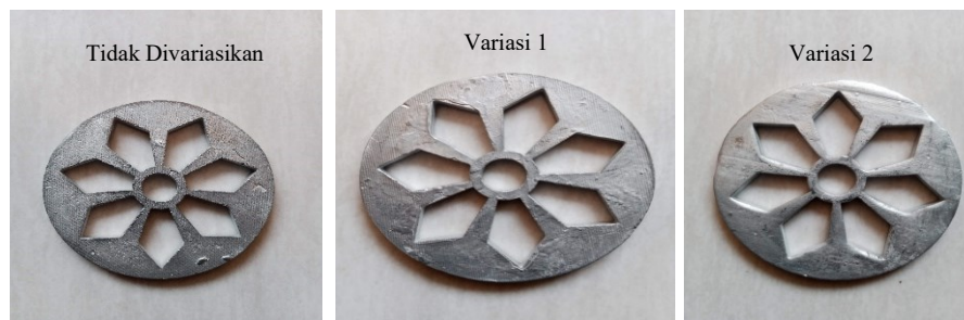
Gambar 4. 15 Hasil Spin Casting 600 RPM Percobaan 1
