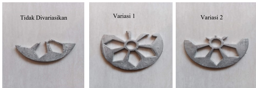
Gambar 4. 11 Hasil Spin Casting 500 RPM Percobaan 1
