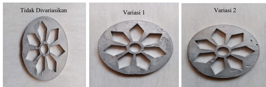
Gambar 4. 12 Hasil Spin Casting 500 RPM Percobaan 2
