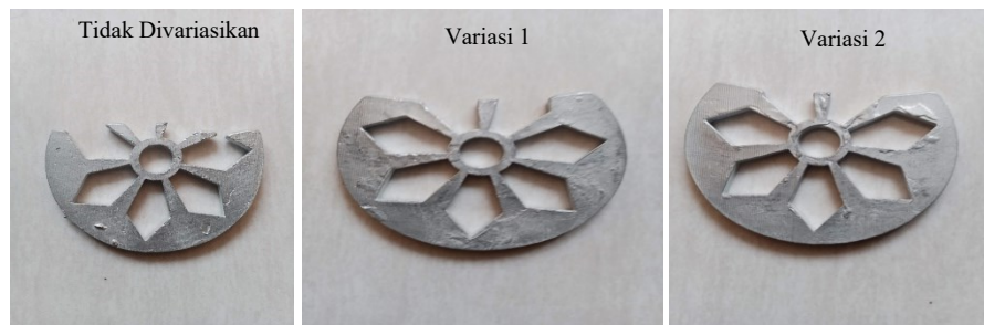
Gambar 4. 19 Hasil Spin Casting 700 RPM Percobaan 1
