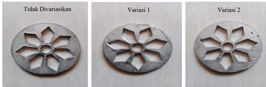
Gambar 4. 13 Hasil Spin Casting 500 RPM Percobaan 3
