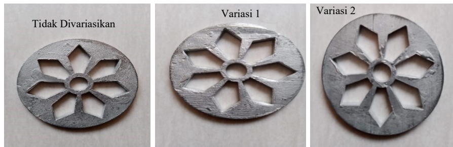
Gambar 4. 26 Hasil Spin Casting 800 RPM Percobaan 4
