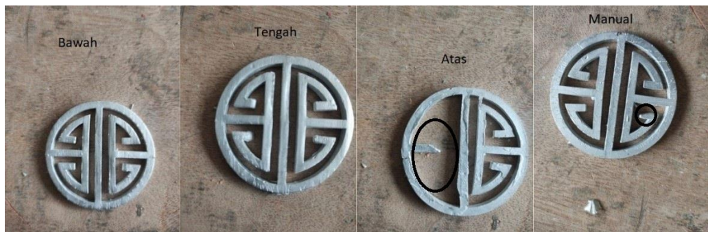
Gambar 4- 14 Hasil Spin casting 900 RPM Percobaan 3
