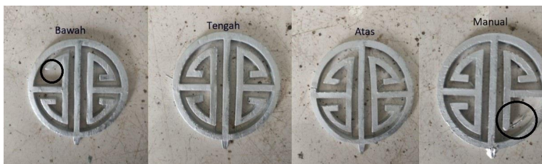
Gambar 4- 6 Hasil Spin casting 800 RPM Percobaan 1
