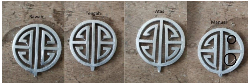
Gambar 4- 10 Hasil Spin casting 850 RPM Percobaan 2
