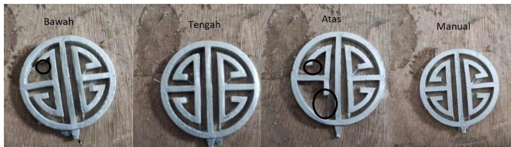
Gambar 4- 8 Hasil Spin casting 800 RPM Percobaan 3
