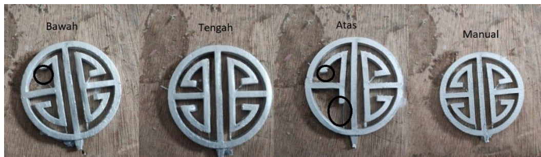
Gambar 4- 9 Hasil Spin casting 850 RPM Percobaan 1
