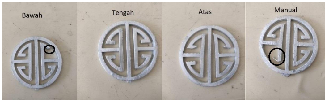
Gambar 4- 7 Hasil Spin casting 800 RPM Percobaan 2
