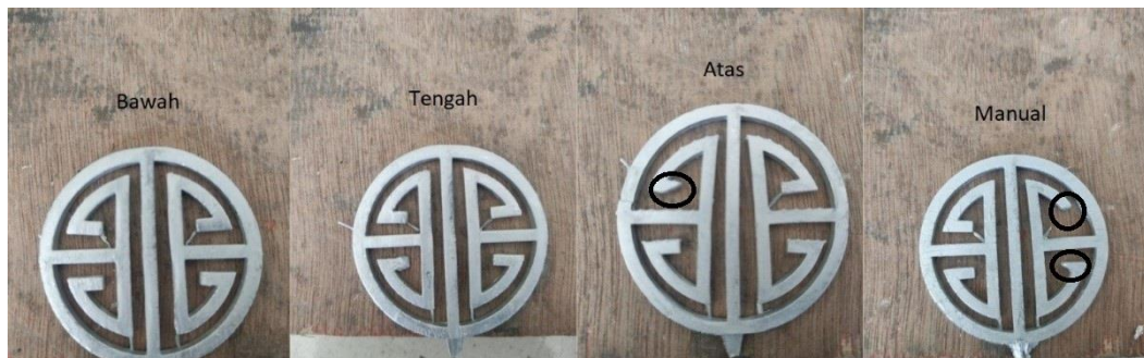
Gambar 4- 11 Hasil Spin casting 850 RPM Percobaan 3
