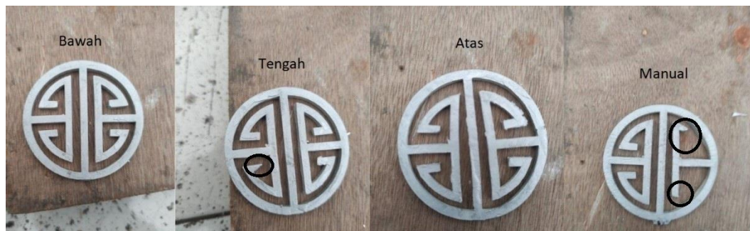
Gambar 4- 12 Hasil Spin casting 900 RPM Percobaan 1
