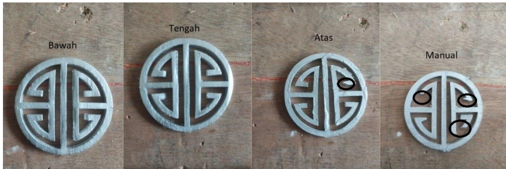
Gambar 4- 13 Hasil Spin casting 900 RPM Percobaan 2
