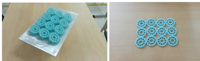
Gambar 4-6 Master Hasil Proses 3D Print Resin
