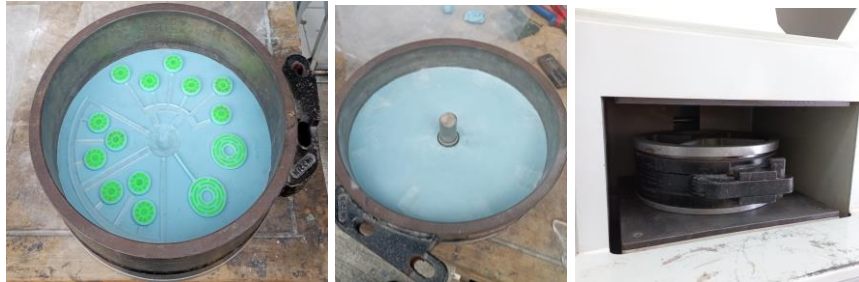
Gambar 4-9 Proses Vulkanisir Silicone Rubber Mold
