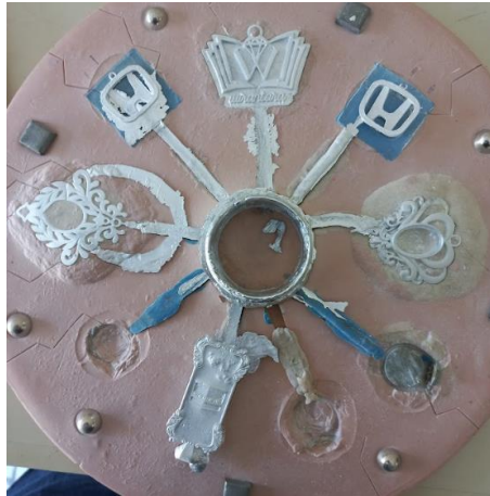
Gambar 4-22 Hasil percobaan spin casting
