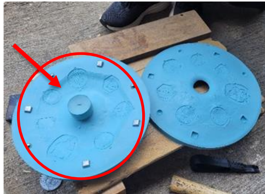
Gambar 4-45 Cacat hasil vulkanisir
