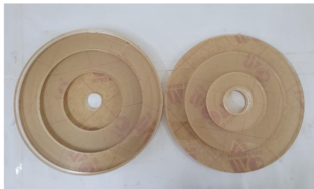
Gambar 4-6 Part hasil laser cutting
