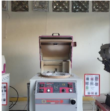
Gambar 4-23 Mesin pelebur material f-120 matic
