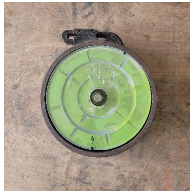
Gambar 4-15 Besi penahan tengah
