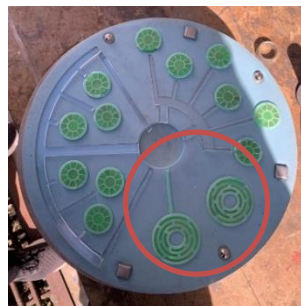
Gambar 4- 13 kondisi master hasil 3D print resin
