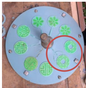
Gambar 4- 14 kondisi master hasil 3D print resin
