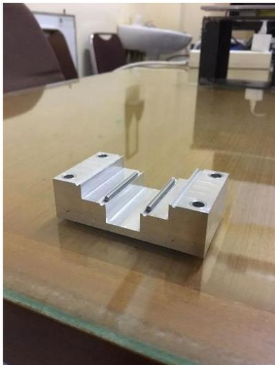
Gambar 3 - 13 Komponen *Support* Hasil CNC
