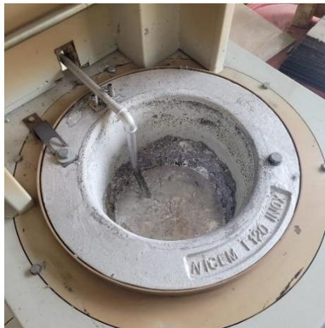
Gambar 4- 12 Proses Peleburan Zinc Alloy
