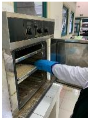
Gambar 4. 10 Bahan Adsorben Sumpit Bekas Dioven Sumber: Data Primer, 2023
