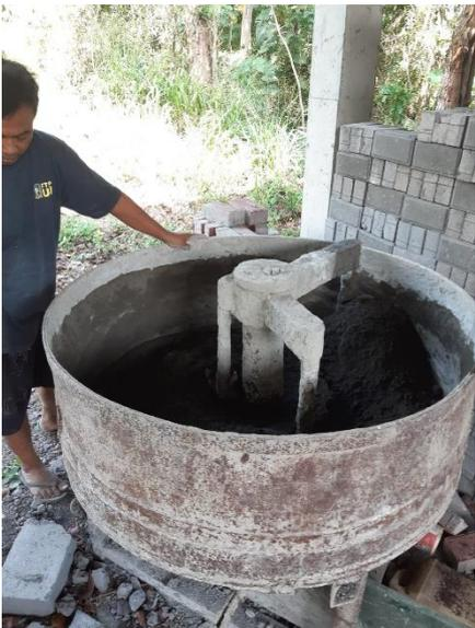
**Gambar 5.11** Proses Mixing Bahan Susun Batako di Mixer Machine
