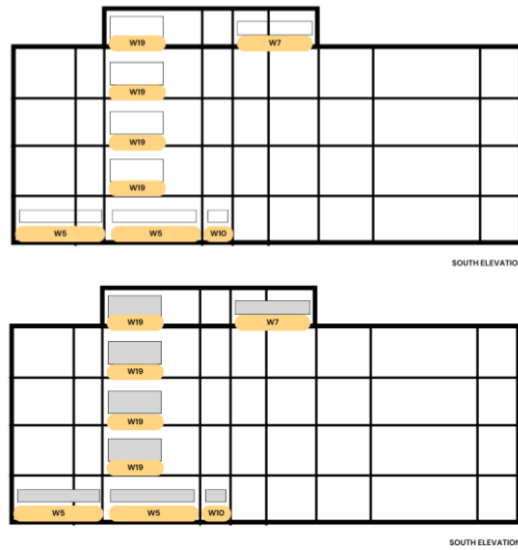
Figure 7 Changes of glass material on the south side, before and after (upper, lower) Source: Author, 2023
