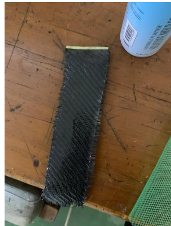
Gambar 3-33 Pelapisan lem ALF epoxy adhesive
