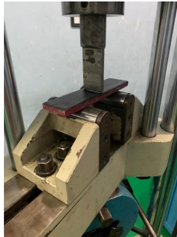
Gambar 4-1 Proses pengujian three point bending
