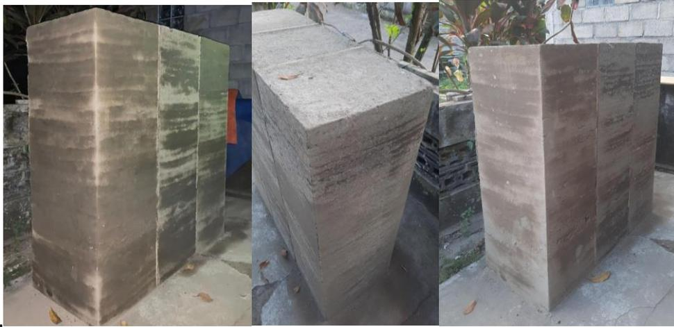
**Gambar 3** *Prototype* dinding tanah
