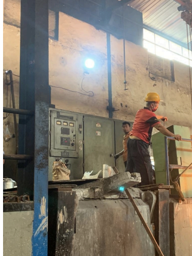
Gambar 4. 7 Memeriksa temperature mesin oven
