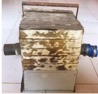
7. Heat Exchanger Box
