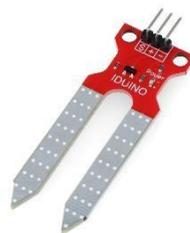
Gambar 2. 5 Sensor Kelembaban Tanah
