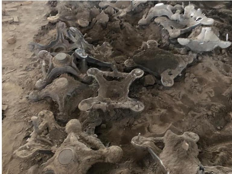
Gambar 4. 6 *Grinding Ball*
