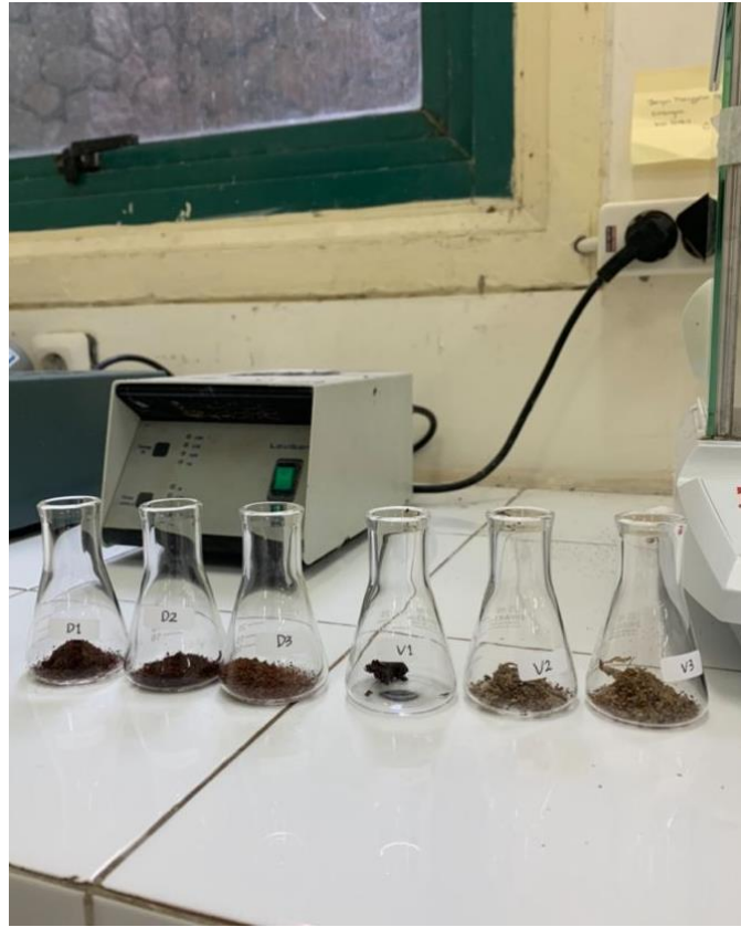
Gambar II. 13 Proses Pengujian C-Organik
