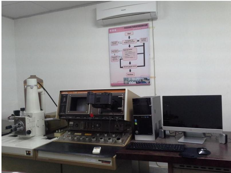
Gambar Instrument SEM
