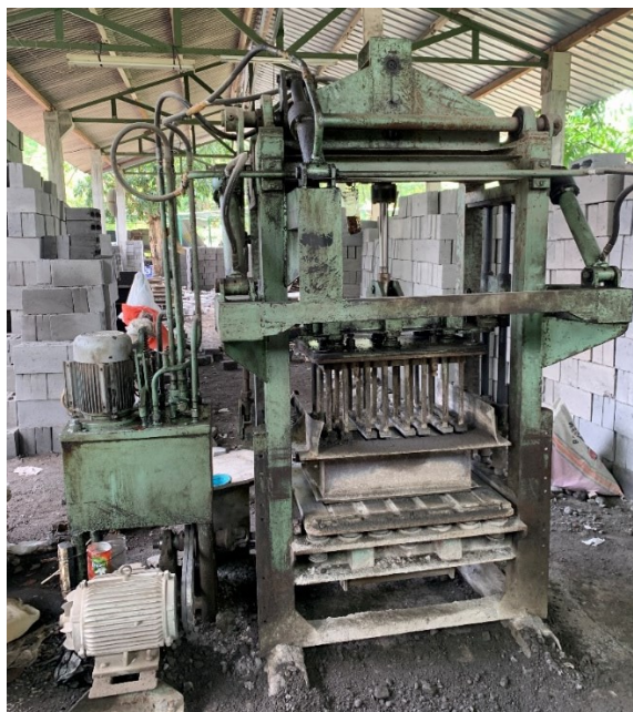
Gambar 4. 6 Mesin Press Paving block
