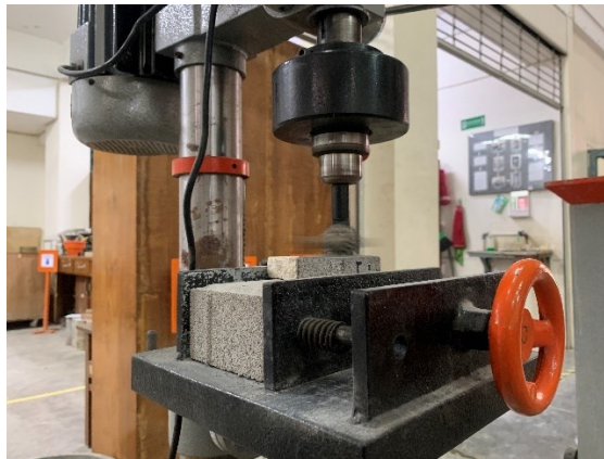
Gambar L-3.4 Uji Keausan Paving block
