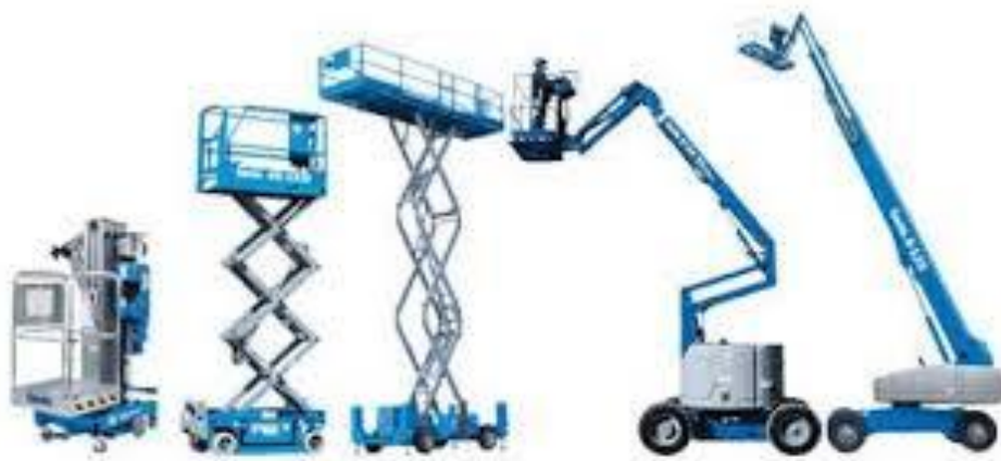
Gambar 3.3. Aerial Lifts Scaffolding
