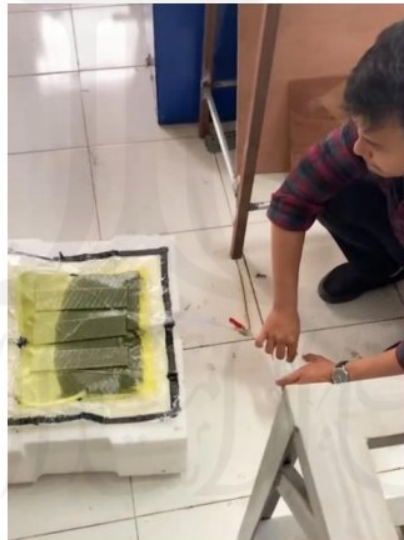
Gambar 3. 27 Proses Vacuum Infusion
