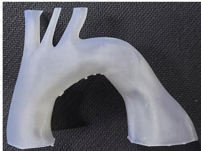
Gambar 4- 30 Hasil Pencetakan 3D Print Thoracic Aortic Aneurysm
