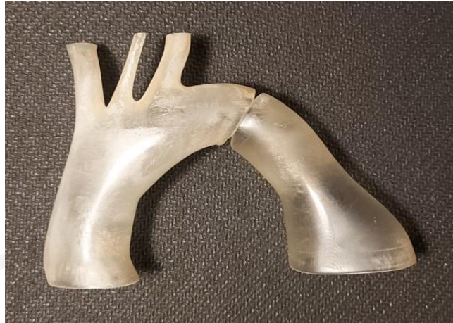
Gambar 4- 35 3-D Printed Model Thoracic Aortic Aneurysm Dibagi 2 Bagian
