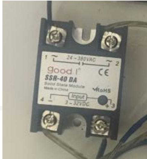
Gambar 4- 16 Solid state relay
