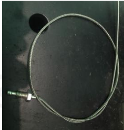
Gambar 2- 3 Sensor suhu Termokopel
