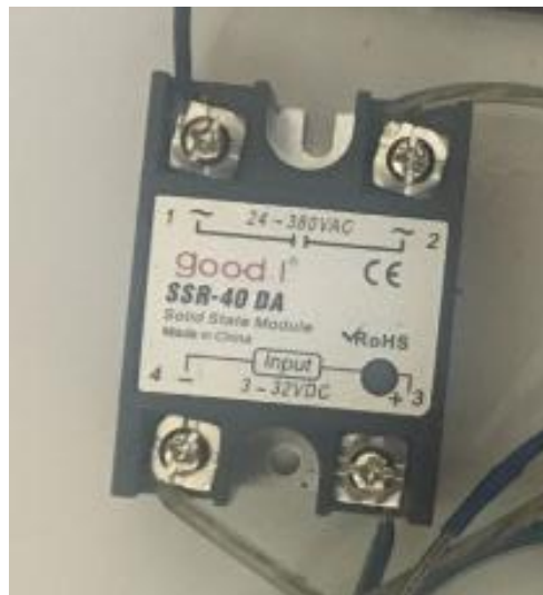
Gambar 2- 5 Solid state relay
