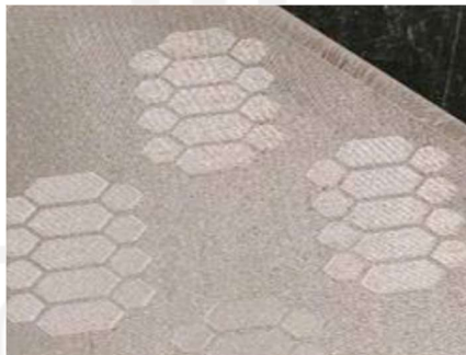
Gambar 2–3 Hasil 3D print sisik perut ular berbahan 420 stainless steel [5].
