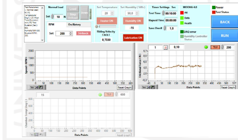
Gambar 4-1 Tampilan antarmuka tribometer pin on disc .
