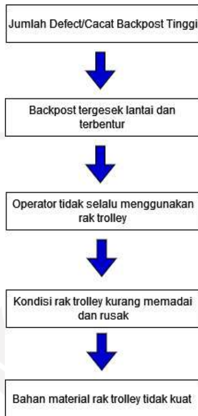
Gambar 4. 10 Defect 5 Why's Analysis
