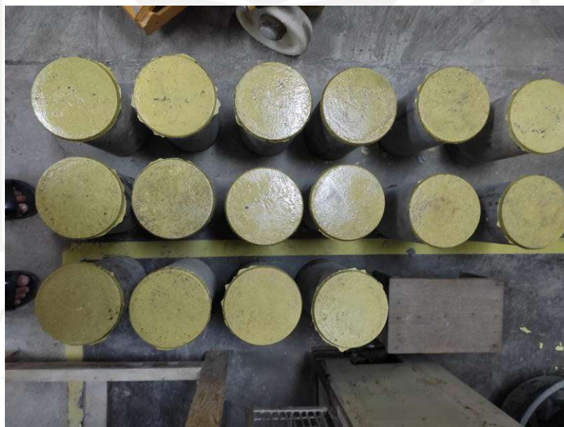
Gambar L-12. 2 Proses capping benda uji silinder
